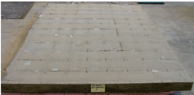
Figure 30. Full height flat-panel ICF with high slump concrete (no mechanical vibration). (IMG13382)
