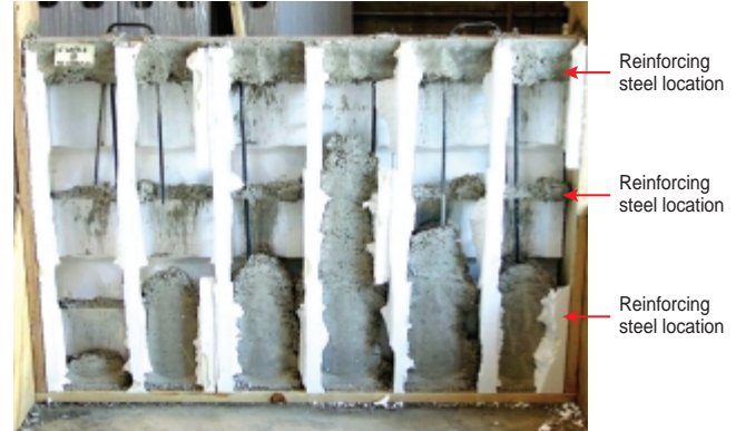
Figure 12. Waffle-grid ICF with low slump concrete and no mechanical vibration. (IMG13344)
