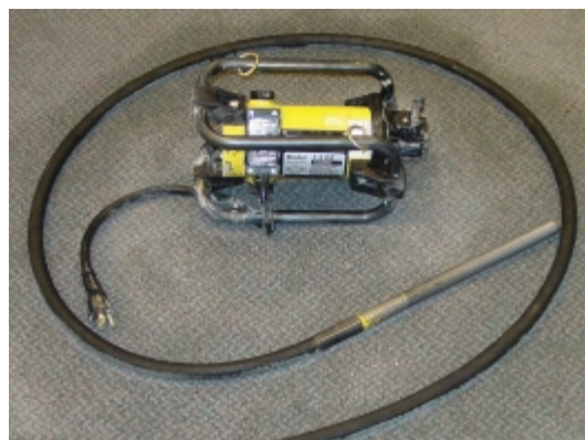
Figure 5. Internal concrete vibrator (disassembled). (IMG13338)
