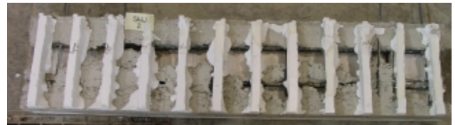
Figure 25. Flat-panel ICF lintel with low slump concrete vibrated with a reciprocating saw. (IMG13371)
